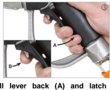
Pull lever back (A) and latch as shown (B). You can remove your hands from the nozzle.
