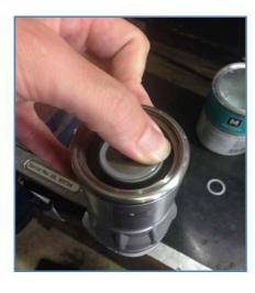
You will feel when the O'ring is completely in the groove as there will be no more lumps. It is important to make a secondary to check to see if the O'ring is flat and not wavy. If uneven push back into groove to flatten out.
