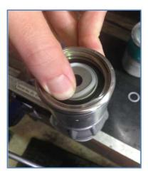
Start the O'ring in the groove of the nose piece by pushing in one side, the lubrication should assist this part of the assembly. Continue to push down on the O'ring and move around the nose piece until the O'ring is completely pushed in.
