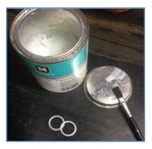
Hold the nozzle upright in a vice by clamping the guard on the nozzle body. Take an oil based lubricant (we recommend Molycote) and apply it sparingly to the surface of the O'ring
