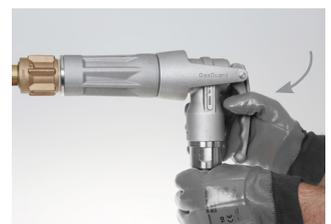
After refueling disengage lever. Prepare for disconnection.
