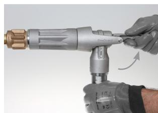
Actuate lever until held in cam open position. Start refueling.
